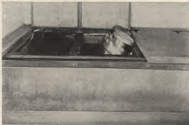
The insulated concrete cooling tank is economical to build and helps cool milk efficiently.
